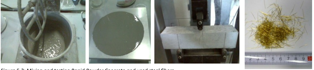
Figure 5.2: Mixing and testing Rapid Powder Concrete and used steel fibers
