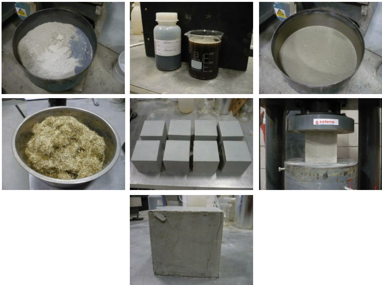
Figure 10.1: Preparing, mixing and testing mix C120
