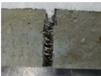
Figure 10.5:sample after testing flexural strength
