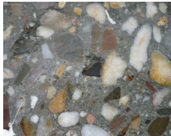
Figure 8.4: Surface of 205 days old concrete with 0,3% ConcreCem after 14 cycles of Freeze-thawing
