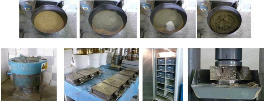
Figure 3.3: Mixing mortar, casting and curing samples and testing
