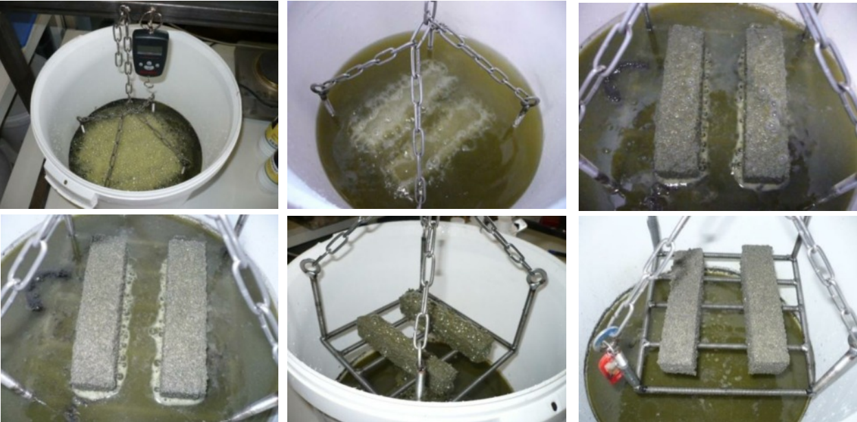
Figure 6.1: Immersion in 36% M hydrochloric acid (pH = 0,45) and deterioration of the prisms
