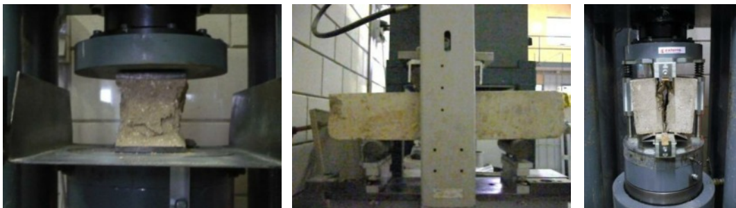
Figure 3.5: Testing compressive strength, tensile strength and tensile splitting strength.
