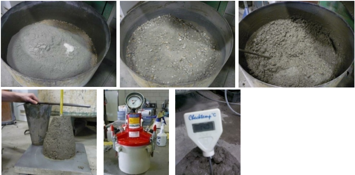
Figure 3.3: Mixing and testing (slump, air content and temperature) wet concrete
