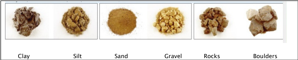
Figure 4.11 Typical appearances of clay, silt, sand, gravel, boulders and rocks.
