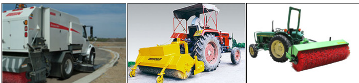
Figure 5.46 Mechanical Surface finishing brooms.
