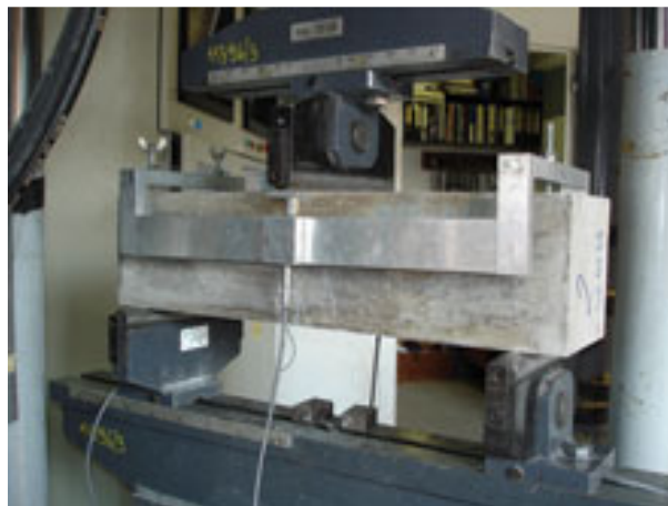
Figure 5.34 Three-point bending flexural test.
