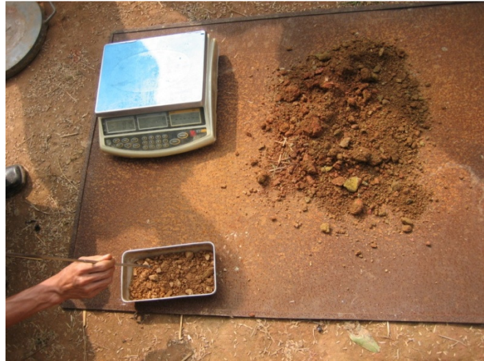
Figure 4.18 Measuring the weight of the samples before packing in an airtight bag.
