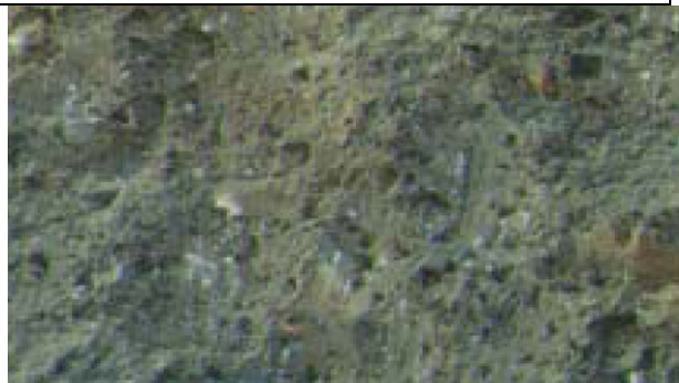
Structureless --Massive: No discrete structural units observable in place or in hand sample. Material is coherent
