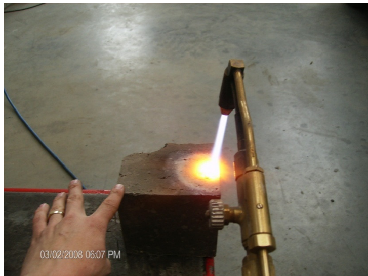
Figure 2.12 Thermal lance on sludge mixed with PowerCem based product.
