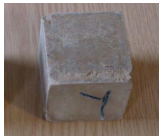
Figure 19. FireCemY cube almost intact after exposure to liquid nitrogen & 6 drop tests
