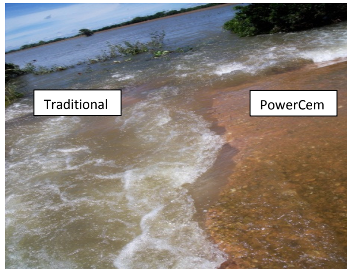
Figure 2: Difference in erosion between traditional pavement construction and RoadCem
